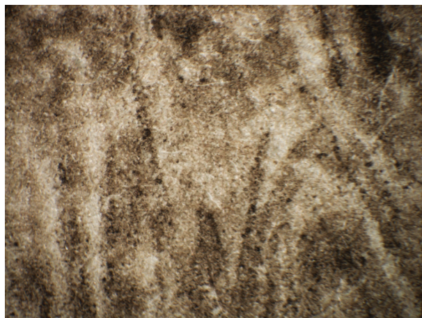
Figure 5b Microscopic structure of the Dmin area of the print in fig. 4a at 25× magnification.
