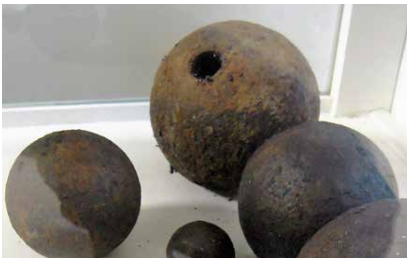
Cannon balls made of iron suffering from corrosion because of high relative humidity (Image courtesy of José Luiz Pedersoli Jr.).
