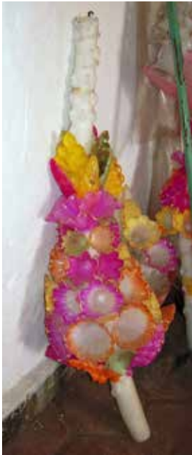
Softening and deformation of a (paraffin wax) candle exposed to higher temperature from direct sunlight while stored leaning against the wall (Image courtesy of José Luiz Pedersoli Jr.).
